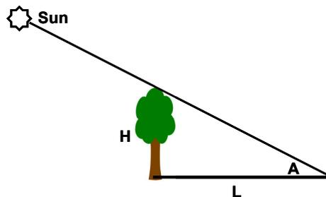
**Figure 1: The basic trigonometry concept for height determination**
